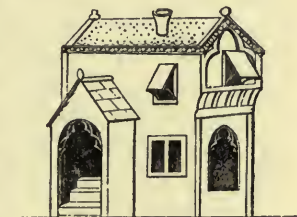
HOUSE WITH EXTERNAL STAIRCASE PROTECTED BY A PORCH
